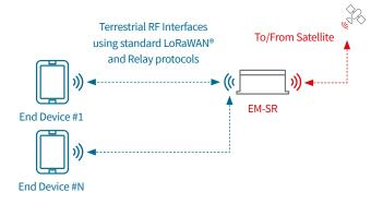
End-devices operating behind the EM-SR must support the relay stack in their software which allows them to use the standard radio protocol defined in LoRaWAN® TS011.
